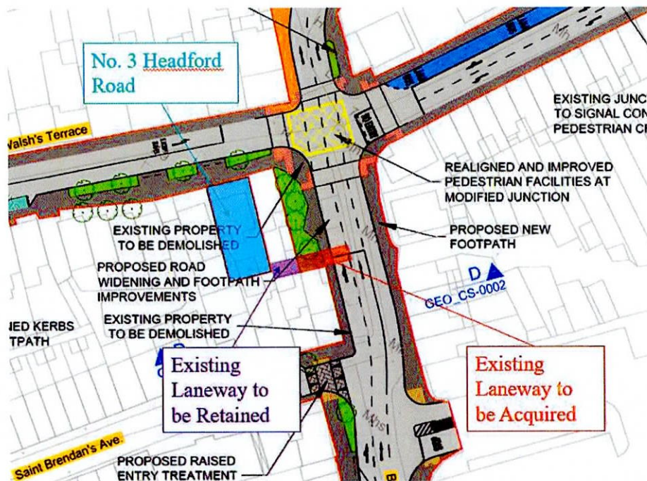
Figure 2.5 – Retained Laneway at No. 3 Headford Road
